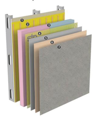
Substrate: Glass Mat Gypsum sheathing in compliance with ASTM C 1177, Exterior or Exposure I wood-based sheathing (plywood or OSB), code compliant concrete, concrete masonry, or portland cement plaster, existing structurally sound, uncoated brick or other masonry wall construction.
